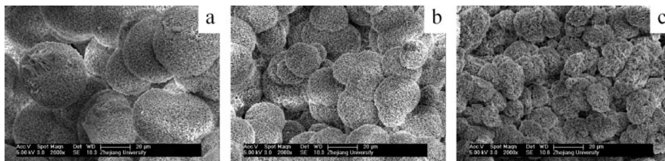
Figure 8 Micrographs of the cross sections of membranes in the system of 100 wt/0 wt DBP/DEHP. Polymer concentration: 30 wt %. Cooling rate: (a) 5°C/min; (b) 10°C/min; (c) 30°C/min.
